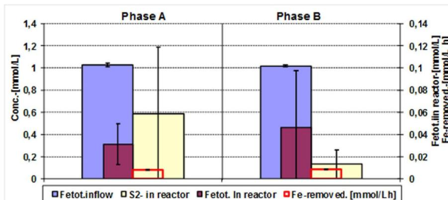
Fig. 6. Relations between iron and iron sulfide concentration and removal rate in the reactor with methanol as a carbon substrate for phase A (HRT of 5.2 days) and phase B (HRT of 4.7 days)
