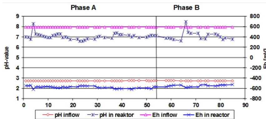
Fig. 5. relationships between redox potential and pH in the reactor with methanol as a carbon source during phase A and phase B
