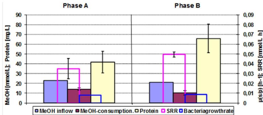
Fig. 4. Relations between methanol and methanol concentration in feed consumption, protein concentration, sulfate reduction rate (SRR) and Bacterial growth rate ( $\mu(s/p)$ ) in phase A and phase B, (hydrogen flow
