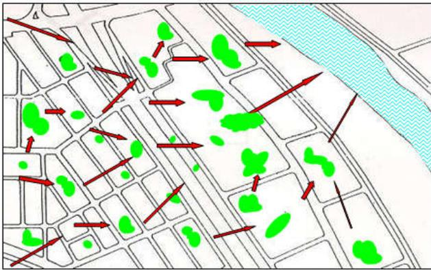
**Fig. 7. Schematic diagram of scattered low-impact runoff retardation facilities (Liaw et al., 2000)**
