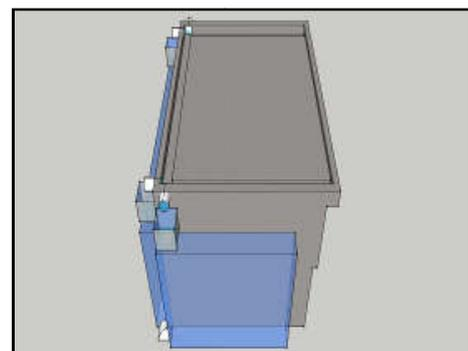
Fig. 6. A newly improved above ground rainwater harvesting scheme using the vertical walls of the residential house
