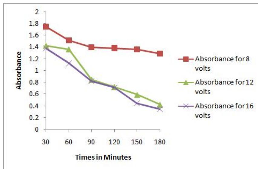
Figure c. Variation of Absorbance with voltage (EC &amp; Aeration)
