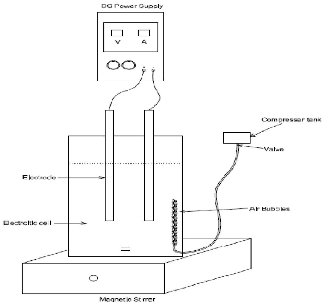
Figure a. Experimental set up of Electro-coagulation with aeration
