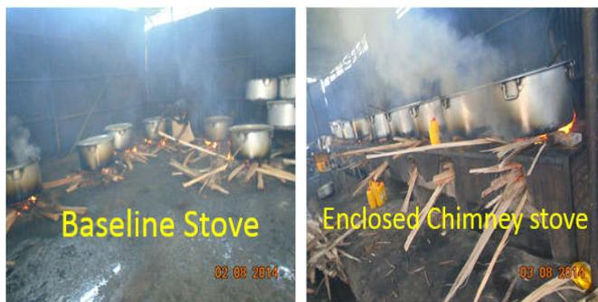
**Figure 1. Enclosed chimney and Baseline stove during operation**
