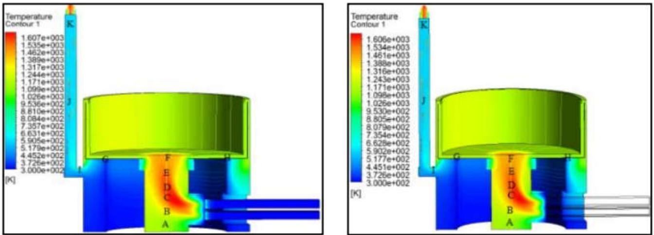
Figure 10. Supplying both primary and secondary air (75% - 25%)
