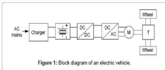
Figure 1: Block diagram of an electric vehicle.
