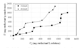
Fig. 2. Influence of NaCl concentration on the adsorption isotherm
