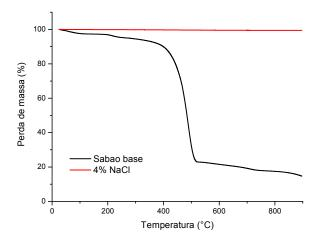
Fig. 5. Loss of mass (%) for pure BS and sandstone with BS and 4% NaCl
