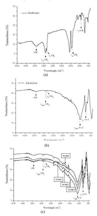
Fig. 3. Transmittance (%) versus wavelength (cm<sup>-1</sup>) to pure BS (a), pure sandstone (b) and sandstone with adsorbed surfactant (c).
