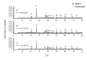
Fig. 4. XRD of pure sandstone (a) of sandstone with BS (b) and sandstone with BS and 4% NaCl (c)
