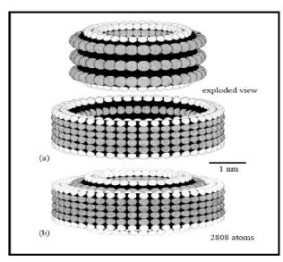
Fig. 3: Exploded view of a 2808-atom strained-shell sleeve bearing.<sup>15</sup> Image courtesy of K.Eric Drexler.© 1992, John Wiley and Sons, Inc.
