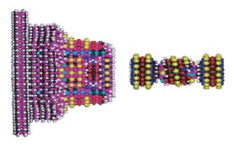
Fig. 5. Side views of a 6165-atom neon gas pump/motor.<sup>19</sup> Image courtesy of K.Eric Drexler. © Institute for Molecular Manufacturing (www.imm.org)
