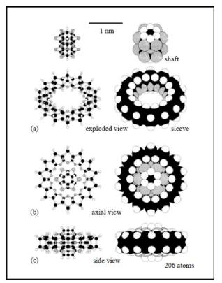
Fig. 2: End views and exploded views of a 206-atom overlaprepulsion bearing.<sup>15</sup> Image courtesy of K.Eric Drexler.© 1992, John Wiley and Sons, Inc.
