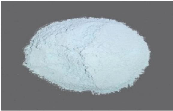
Figure 1. Copper oxide nanoparticles loaded Zeolite
