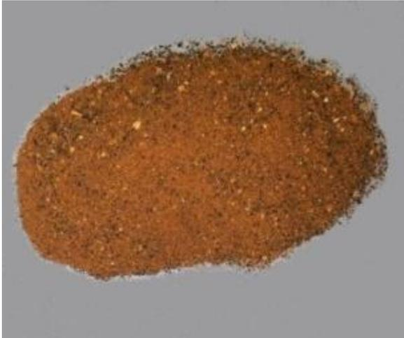
Figure 2. Iron oxide nanoparticles loaded Zeolite
