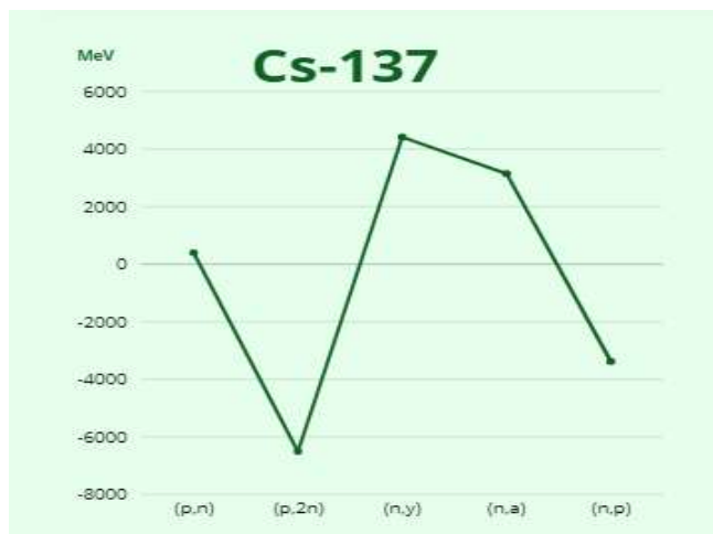
Figure X. Q-value of the nuclear reactions studied for the target formed by the radioisotope Cs-137
