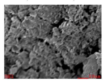
Figure 5. Show the composition of rice husk briquettes graph using an SEM after the distilation process
