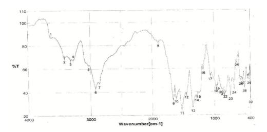
Fig.1. Infra red spectral of N 15 Phenothiazine derivative
