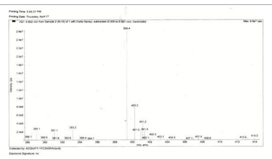
Fig. 3. Mass spectra of N15 compound
