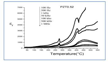
Figure 7. Spectrum of the dielectric constant of the sample PZT52 depending on the temperature
