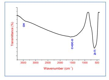
Figure 3. IR spectrum of the sample PZT52
