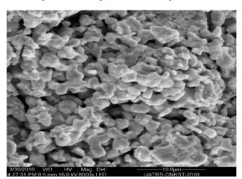
Figure 6. SEM image of a pellet sintered at 900 °C for 4 hours of sample PZT52
