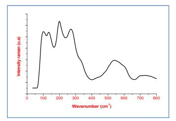
Figure 5. Raman spectrum of the sample PZT52
