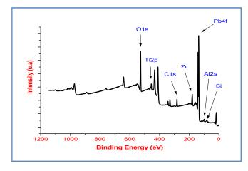
Figure 8. XPS spectrum analysis of the sample PZT52
