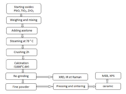
Figure 1. Flowchart of procedure used in the preparation of PZT sample
