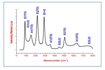
Figure 4. Raman spectrum of the sample PT
