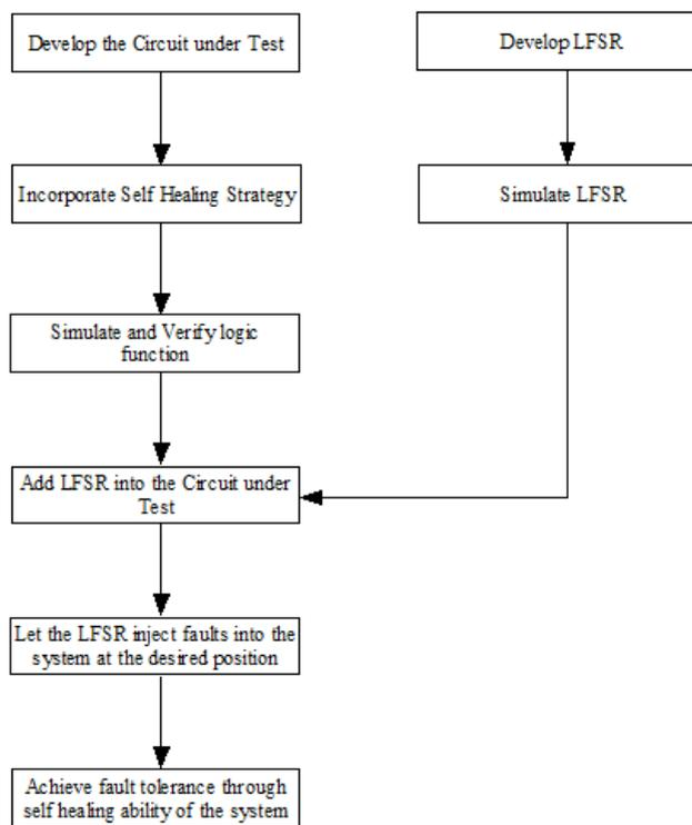
Fig. 3. low diagram of the fault tolerant design
