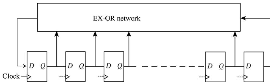
Fig. 1 Block diagram of the self healing decoder
