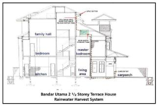
Fig. 5. Rainwater Harvesting System in Bandar Utama
