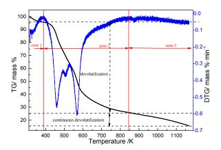
Fig. 1. TG and DTG of NOR with 1K/min
