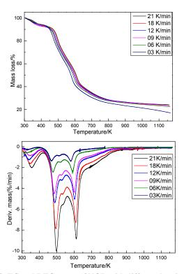
Fig. 2. TG and DTG curve of NOR with different heating rates
