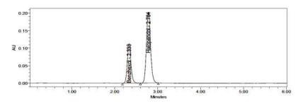
Figure 3 (b). RP-HPLC Chromatogram of Benzhexol and Haloperidol Formulation
