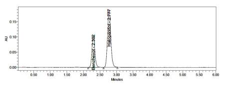
Figure 3 (a). RP-HPLC Chromatogram of Benzhexol and Haloperidol
