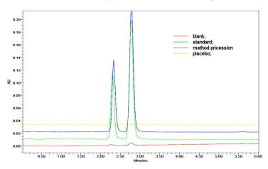
Figure 3 (c). Specificity overlay chromatogram of blank, standard, placebo and marketed sample of Haloperidol and Benzhexol
