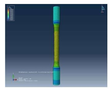
Figure 7. Stress with pores
