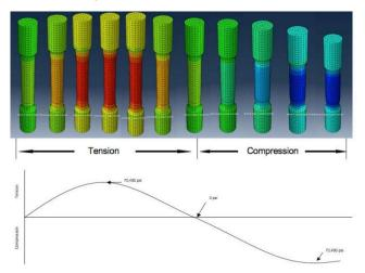
Figure 9. Reverse Loading: Cavity test specimen
