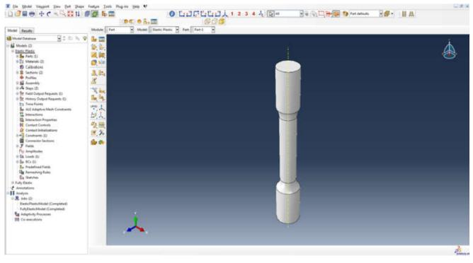
Figure 2. Created part revolved around center line
