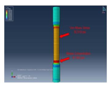
Figure 5. Von Mises Stress Figure
