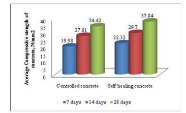
Figure 3. Comparison of Compressive strength of Controlled and Self healing concrete
