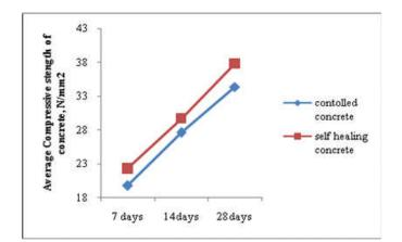
Figure 2. Comparison of Compressive strength of Controlled and Self healing concrete
