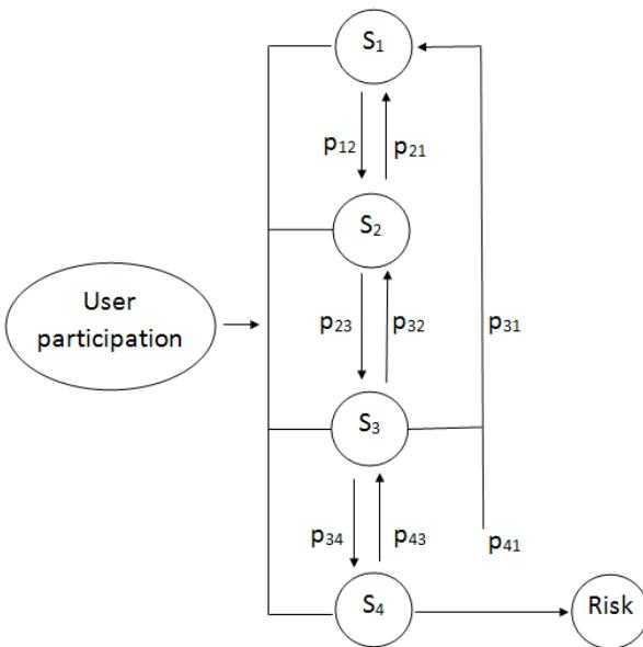
**Figure 3. Model of State Transition diagram for the Unified Process – UP**
