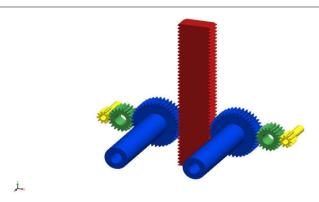
Fig 4. Double sided Rack and Pinion arrangement
