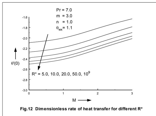
Fig.12 Dimensionless rate of heat transfer for different R\*
