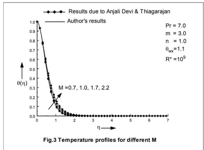
Fig.3 Temperature profiles for different M
