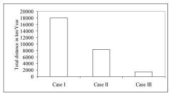
Figure 2.0. Total Distance Traveled by the Vehicle for Collection of MSW in Singanallur Ward for Various Cases
