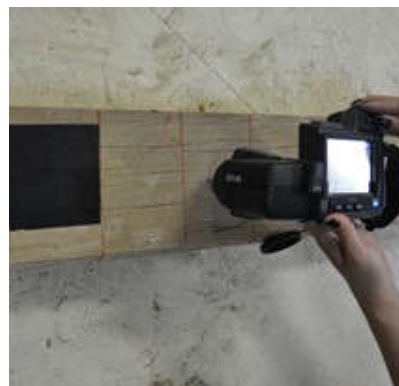
Figure 4. Black body test for determination of emissivity
