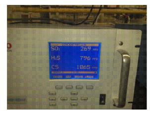
Figure 3. Thermo Electron Corporation 450i H<sub>2</sub>S/SO<sub>2</sub> gases analyzer
