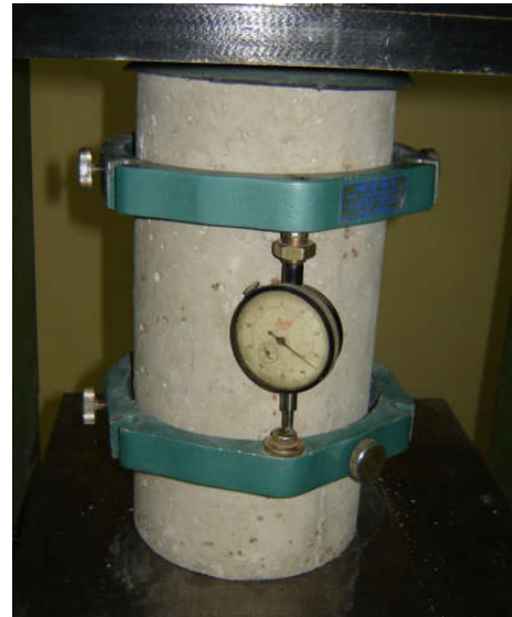
Figure 3. A \phi 15 \times 30 cm cylindrical concrete specimen being subjected to pressure test
