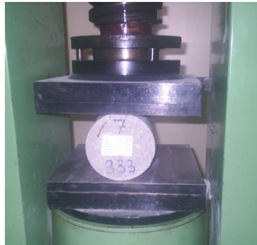
Figure 4. A \phi 15 \times 30 cm cylindrical concrete specimen being subjected to splitting test
