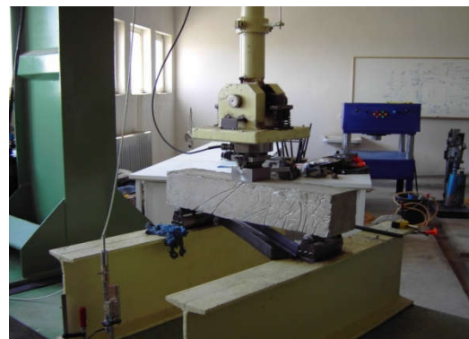
Figure 5. A 15x15x75 cm beam concrete specimen being subjected to bending test
