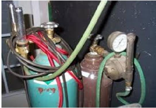
Figure 3. Shielding Gas Cylinder and Regulator
