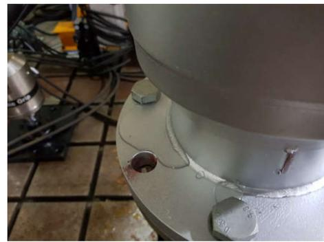
(c) Leakage under durability test
