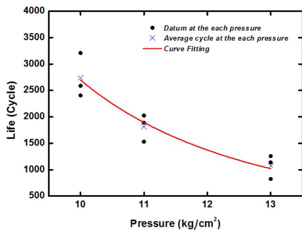
Fig. 5. Curve fitting for datum at each pressure
