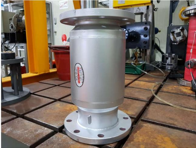
Fig. 1. Specimen: Bellows type expansion joint
