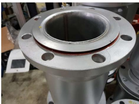
(b) Separation from flange part (breakage)
