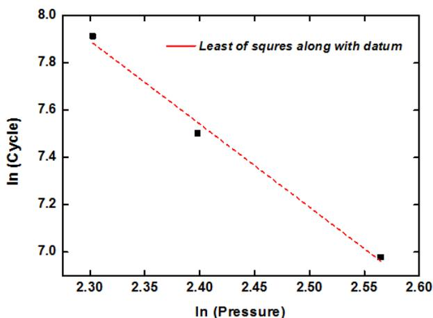
Fig. 8. Conversion into linear transformation of failure lifetime in accordance at 20°C and pressure condition
