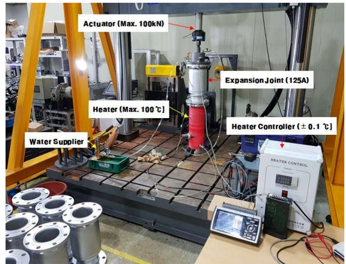
Fig. 3. Set-up for durability test of expansion joint using field data
