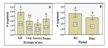
Figure 6. Average of phosphorus concentrations under different use of system (A) and sampling period (B), Santa Barbara, PA. Columns with the same letter do not present statistical difference by 5% Tukey test
