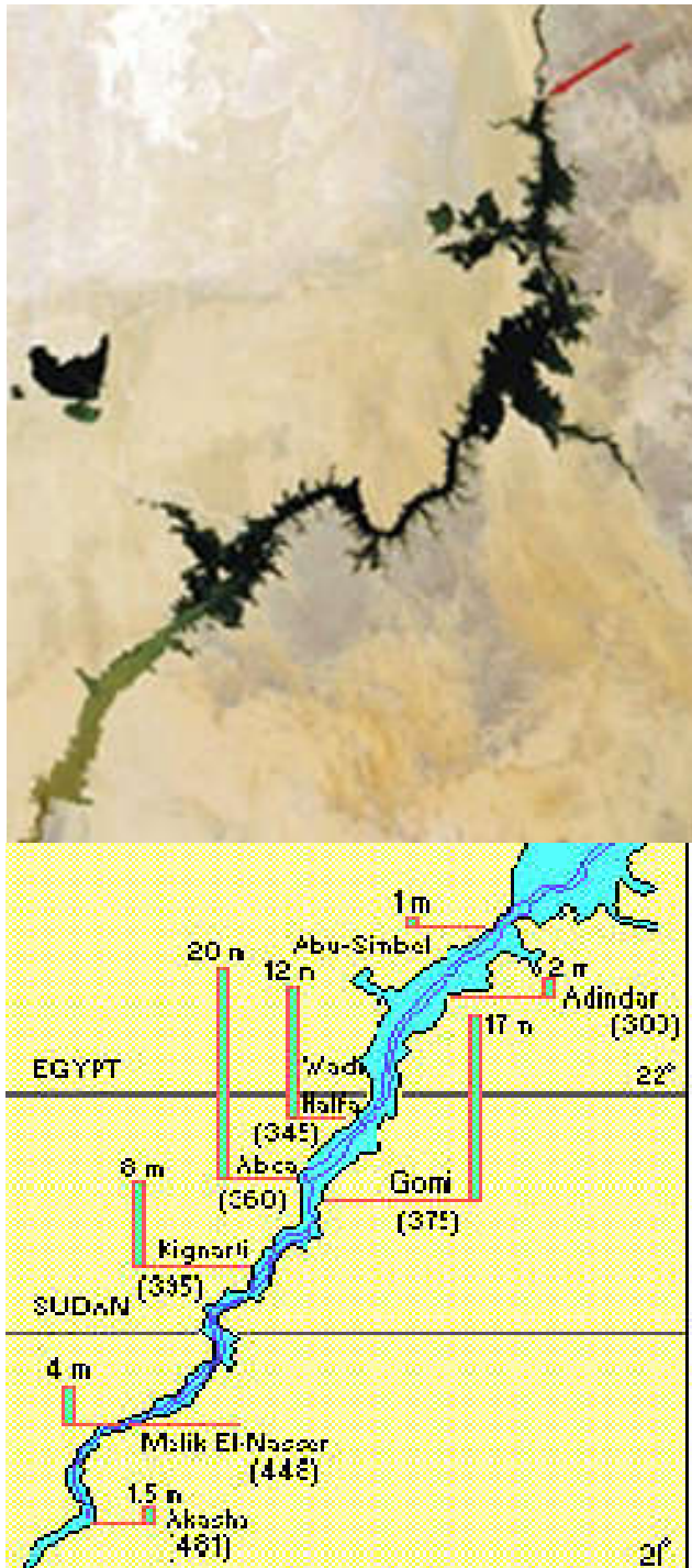
Fig. 2. Distribution of Sedimentation Depth in AHD Reservoir (m) (UNESCO, 2008)
