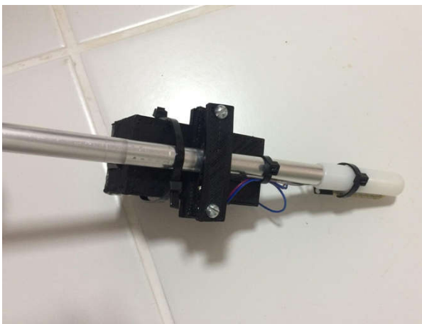
Figure 5. Electronic identifier for moisture detection attached to the extremity of a foldable cane. Campo Grande MS- 2019
