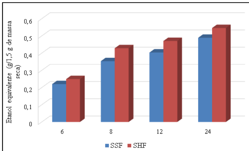
Figure 6. Ethanol production obtained from the release of carbon dioxide (CO 2 ) during fermentation processes (SSF and SHF) from media from pretreated hydrolysate
