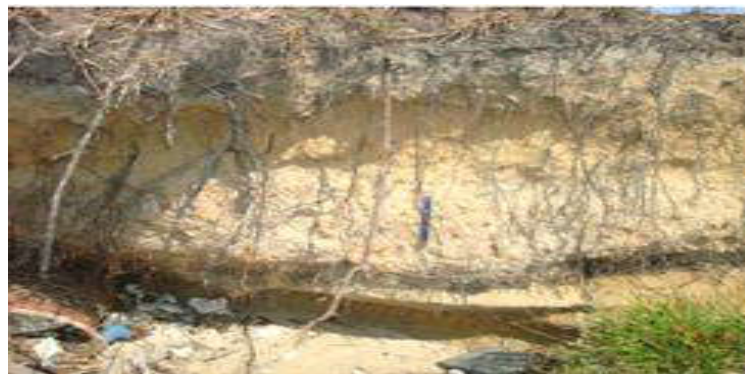
Figure 8. Photo showing in detail the erosion at the edge of the Guamá River at UFPA, making the illustrative comparison with a pen in the center. Source: authors
