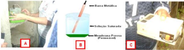
Figure 11. A - Photo illustrating the electrode immersed in a saturated copper sulfate solution. B - Illustrative scheme. C - Voltmeter used in the survey.
