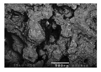
Figure 12. General microstructure of the mortar by SEM. Notably porous area. Secondary electron image (SEI) of the fracture
