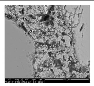
Figure 9. Detailed microstructure of the mortar by SEM. Backscattered electron image (BEI) of the polished section
