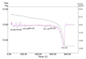
Figure 7. Differential Thermogravimetry (DTG) of the samples of mortar
