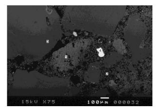
Figure 10. Mortar microstructure by SEM showing big particles of coarse quartz sand and the thin matrix. Backscattered electron image (BEI) of the polished section
