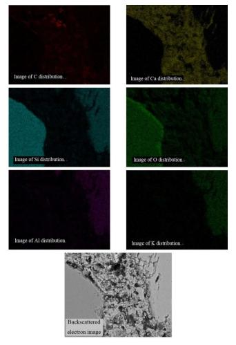
Figure 13. Area mapping of the matrix connecting two large particles (the same area of Figure9)
