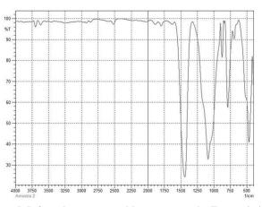
Figure 5. Infrared spectrum - old mortar sample. Transmission method with KBr tablet
