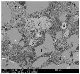
Figure 8. General microstructure of the mortar by SEM. Backscattered electron image (BEI) of the polished section
