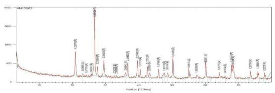
Figure 4. X-ray diffractogram of the old mortar
