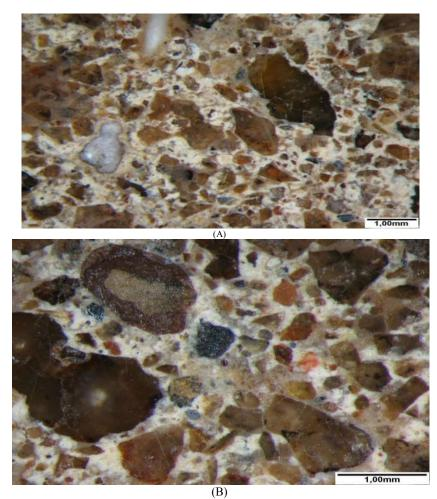
Figure 3. Images ofstereoscopic optical microscope: (a) polished section 1 and (b) polished section 2
