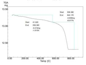
Figure 6. TGA of the samples of mortar, with the losses of mass indicated
