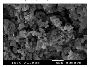
Figure 11. Detailed microstructure of the mortar by SEM, focusing on the thin matrix. Secondary electron image (SEI) of the fracture
