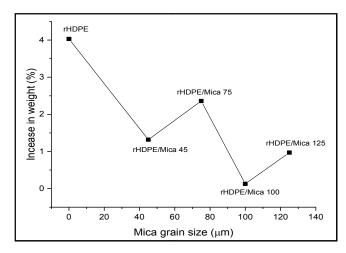
Figure 5. Effect of particle size on the absorbed water of rHDPE/mica composites
