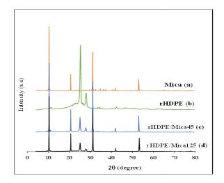
Figure 2. X-ray diffraction patterns of mica (a), rHDPE (b), and rHDPE/Mica45 (c), rHDPE/Mica125 (d) composites
