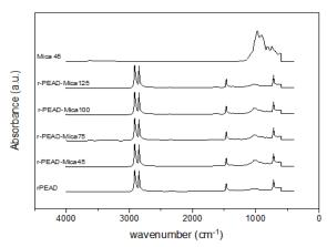
Figure 3. FT-IR spectra of mica, rHDPE and rHDPE/mica formulations
