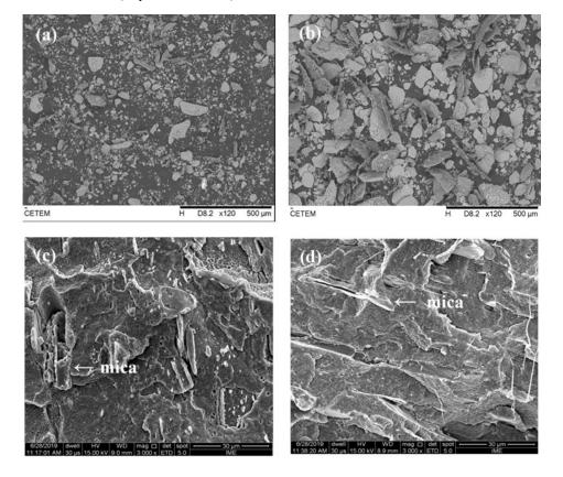
Figure 1: SEM micrographs of mica 45 µm (a), mica 100 µm (b) and fractured surfaces of rHDPE/mica75 (c) and rHDPE/mica100 (d).
