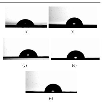
Figure 4. Images of ontact angle with water for: (a) rHDPE, (b) rHDPE/Mica 45, (c) rHDPE/Mica 75, (d) rHDPE/Mica 100 and (e) rHDPE /Mica 125
