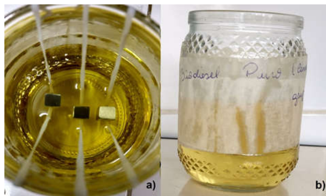
Figure 1. Steel test coupons immersed in biodiesel: a) upper image of the sample, b) frontal image of the sample
