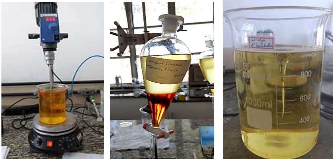
Figure 2. Synthesis of canola biodiesel a) Reaction b) Phase separation: biodiesel and glycerol c) Final Product
