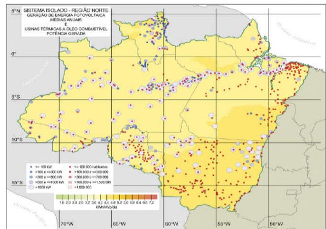
Figure 10: Potential available for daily generation PV in kWh/kWp, in the Amazon region (57).
