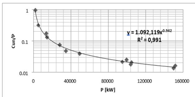
Figure 7: Curve for determining the unit cost of a Brazilian wind farm (51).
