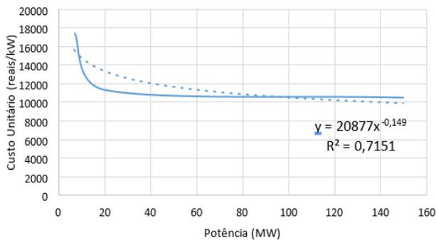
Figure 6: Graphic unit cost as a function of power (49).
