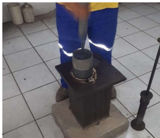
Figure 10. Compaction of the Specimens. Source: The Authors (2020)
