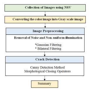
Figure 1. The study approach for detecting the fatigue cracking
