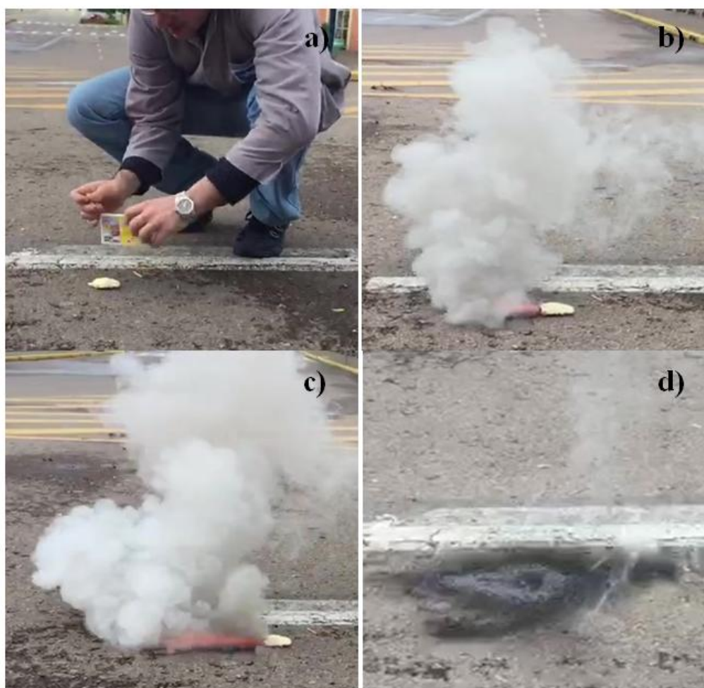
Figure 2. Process of firing rocket fuel before ignition (a), 1s after ignition (b), 2s after ignition (c) and 5s after ignition (d)
