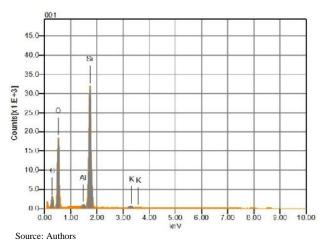
Figure 4. Analysis of the components of a sample of the first micronized ash in Scanning Electron Microscopy (SEM) in the form of ray spectroscopy with a magnification of 700 times
