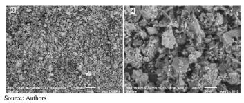
Figure 3. Images produced by Scanning Electron Microscopy (SEM) of samples from the second batch of RHA in its composition enlarged (a) 100 times and (b) 700 times
