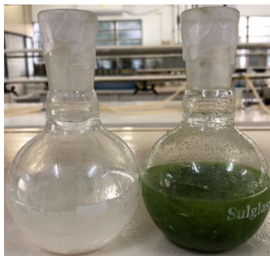
Figure 6: Photo of the prepared samples, with the latex solution on the left side and the crushed branch solution on the right side
