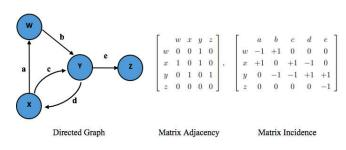
Figure 3. Directed graph used to represent directions of traffic on roads
