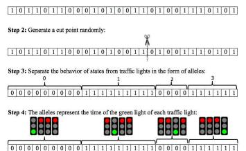
Figure 10. Processing of the genetic algorithm to find the most optimized selection of the traffic light based on vehicle traffic data observed in the field
