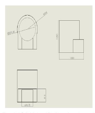
Figure 1- a) Cylindrical type kiln with opening at the top and front "box" b) Side, front and top view of the kiln with main measurements
