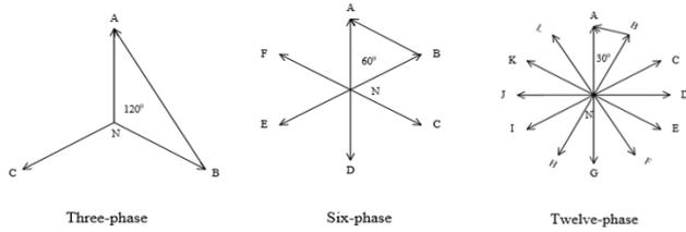
Fig. 1. Three-phase and HPO systems phasors
