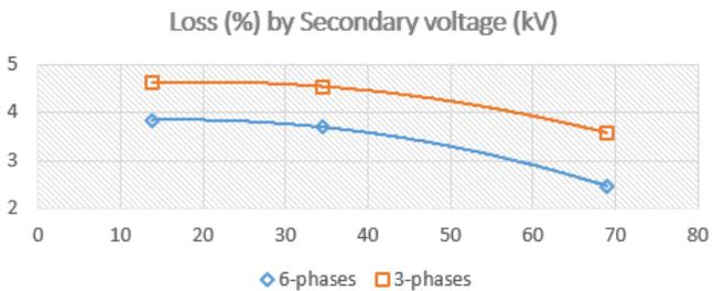
Fig. 6. Simulation changing the secondary voltage
