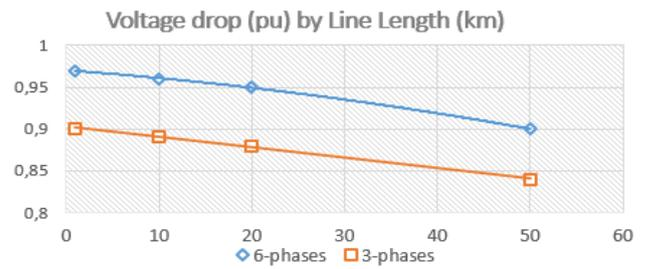
Fig. 5. Simulation changing the line length– $V_{min}$
