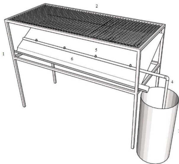
Figure 1. Aeroponic system prototype with one seedling of genotype BD-9 and one seedling of genotype BD-16 of sweet potato ( Ipomoea batatas ), State University of Ponta Grossa (UEPG), Paraná – Brazil, 2019
