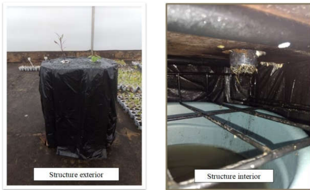
Figure 1. Aeroponic system prototype with one seedling of genotype BD-9 and one seedling of genotype BD-16 of sweet potato ( Ipomoea batatas ), State University of Ponta Grossa (UEPG), Paraná – Brazil, 2019
