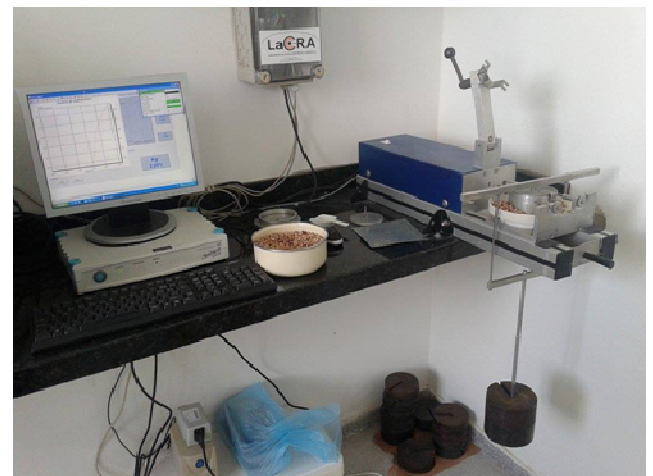
Figure 2. Jenike equipment used to determine flow properties
