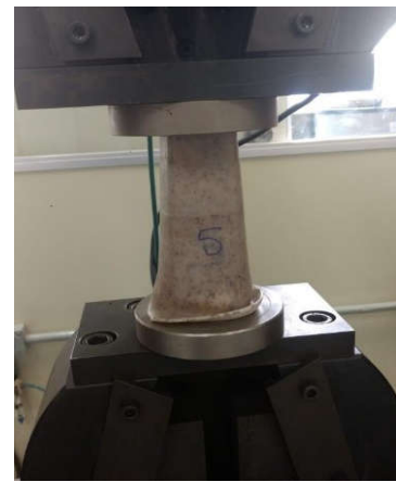
Figure 3. Sample for the compression test
