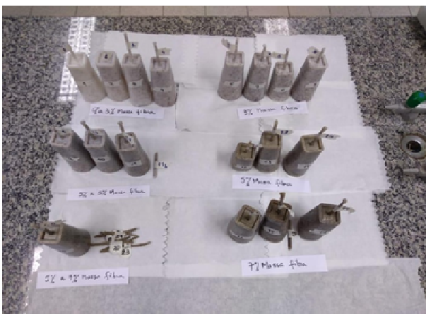
Figure 1. Cups produced from bicomposite (polyethylene + natural fibers).
