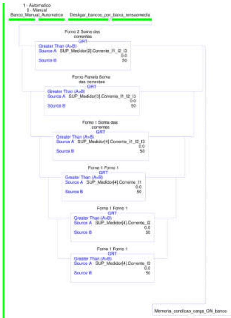
Fig. 12. Controllogix –Load Furnace (Eletric current >50A) – (Author)
