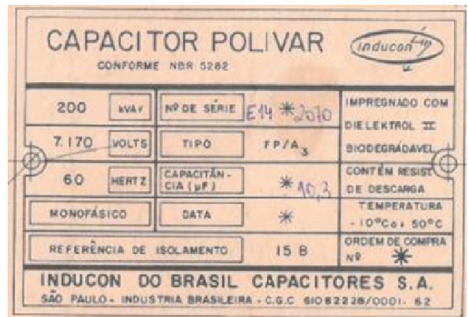
Fig. 2. Capacitor plate data of banks [Author]
