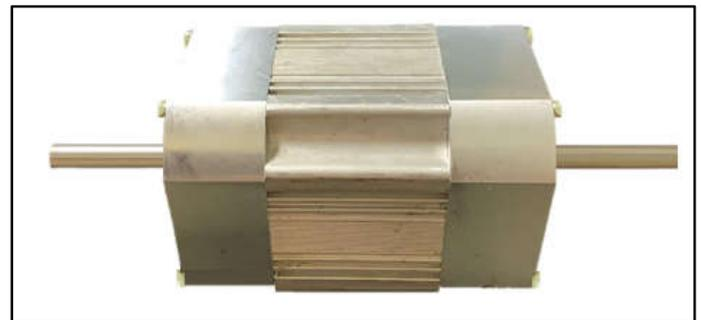
Figure 3. Final assembly of the servomotor
