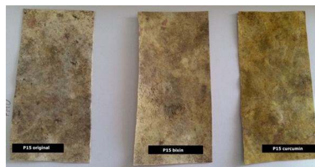
Figure 9. P15 samples after 180 days in free biodegradation test
