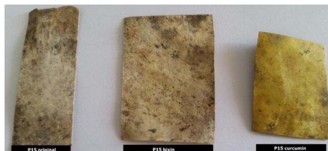
Figure 8. P15 samples after 14 weeks on Bartha respirometry
